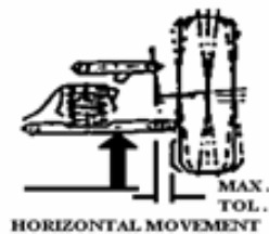
SPRING OR TORSION BAR ON LOWER CONTROL ARM RAISING POSITIONS FOR SUSPENSION SYSTEMS
